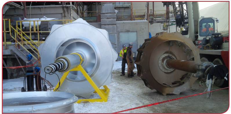
Above: New backward-curved-blade rotor is larger and much more efficient than the old radial-tip-blade rotor.
