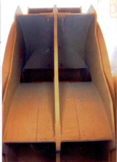
Figure 2 (below): The original fan rotor in 2004. The lack of sufficient wear protection was a primary factor in its failure.
